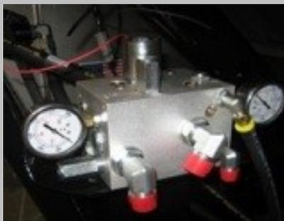
The new hydraulic block shown here, has many benefits over the old system. A hydraulic issue can be diagnosed quickly with pressure & return gauges. Relief port to protect fan motor if too much pressure is applied. Along with relief port is an alarm to notify operator. Replaceable pwm solenoid, convenient and less expensive to replace. Also with the block is an Eaton piston style fan motor. Can upgrade to block (K-0040) with old pwm valve.
