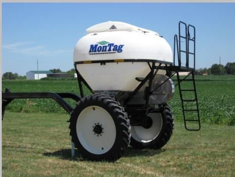
Some of the advantages of the new deck are a portion of the hand rail folds out of the way to allow for easier filling of the tank. The ladder is now mounted with a solid hinge point and when it is folded-up in the closed position it is held
