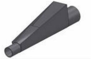
**The Hooded Vent Air Release** has a cover and tube that directs the air and any fertilizer dust in a rearward and downward direction. It can also be fitted with a short piece of tubing (no longer than 36") to further direct the air and dust away from the toolbar and tooling. If a fertilizer tube should plug the fertilizer would be exhausted down with the air.
