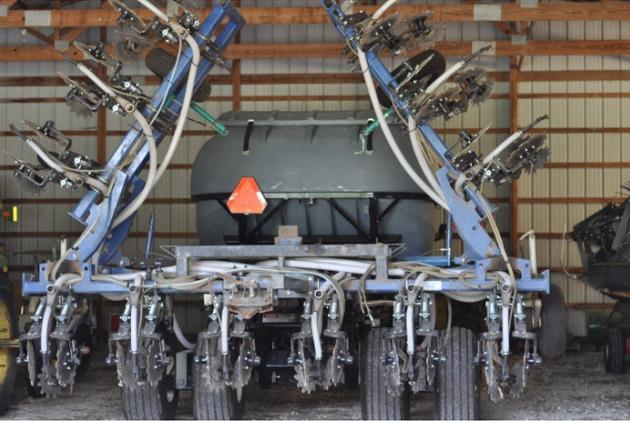
**DRYING OUT. Bland added a mounted Montag dry-fertilizer cart on his Blu-Jet strip-till rig for fall 2013 and will variable-rate a combination of potash and diammonium phosphate in the strip. Moving away from liquid fertilizer application in the fall has been more economical and efficient for Bland.**
