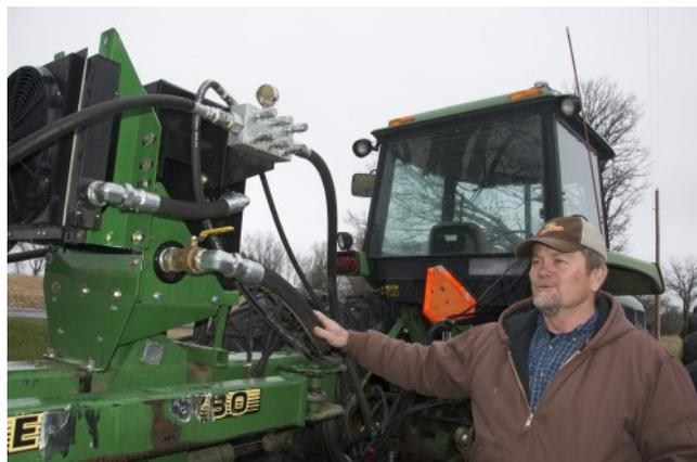
**IMPROVING FLOW.** While Sweeney’s 2-wheel-drive Deere 4755 tractor is able to pull his homemade strip-till unit just fine, he had to enhance the hydraulic flow to run the fertilizer delivery system by installing a Command Hydraulics HydraBoost system on the tractor hitch to provide enough hydraulic capacity to blend fertilizer into the strips.
