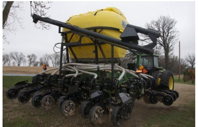
**EQUIPPED FOR SUCCESS.** Edgerton, Wis., strip-tiller Alan Sweeney built a 12-row, 30-foot strip-till rig with second-generation Dawn Pluribus coulter row-units mounted on a old John Deere 1780 planter bar. He also added a Montag Mfg. dry fertilizer bin and attached a fertilizer auger on the back of the rig.
