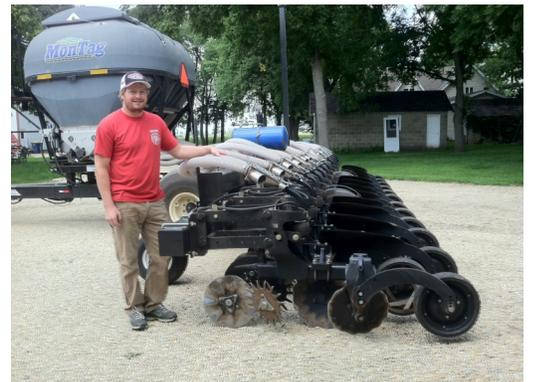
**FERTILIZER FLEXIBILITY.** This spring, Nerstrand, Minn., strip-tiller Nate Bonde added a Montag twin-bin dry fertilizer cart to his family's 12-row strip-till rig and applied 300 pounds per acre of urea and a 75-pound-per-acre mix of monoammonium phosphate (MAP) and sulfate of potash (SOP).
