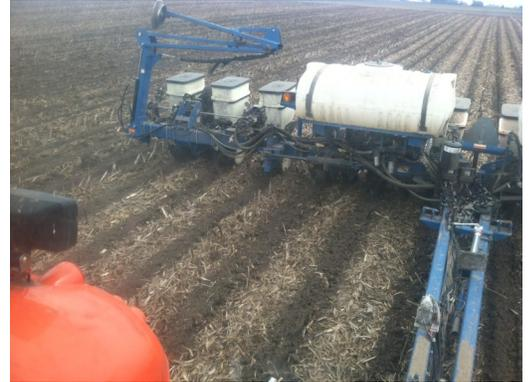
**PRECISE PLANTING.** The Bondes build their strips in spring prior to planting with a 12-row Kinze 3200 planter. In the past, they've sidedressed 4 gallons per acre of 32% nitrogen, but plan to refine fertilizer application through grid sampling in 4-acre plots.
