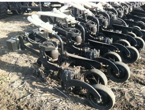
**SUCCESSFUL COMBINATION.** Since moving from ridge-till to strip-till, the Bondes have used Dawn Pluribus row units to build spring strips, but for the first time last fall, also ran a six-row DMI 2500 no-till ripper to help the soil dry out faster in spring.
