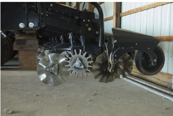
**FITTING THE FIELD.** To accommodate his heavy soils, Duwe prefers a coulter system, rather than a mole knife unit for spring strip-till. Two angled coulters in the back stir the seed zone, and then two gauge wheels with inside blades fluff the strip and prevent clumping.
